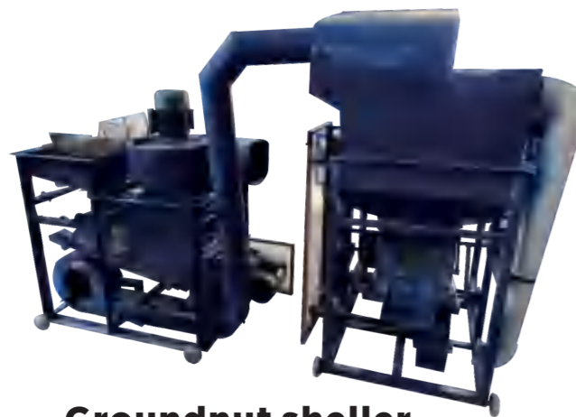
Groundnut sheller BGS-1001 Power:7.5KW/10Hp Weight:600 kg Capacity:300-500Kg/H
